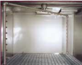
(Standard) Rotating blast pipe system
